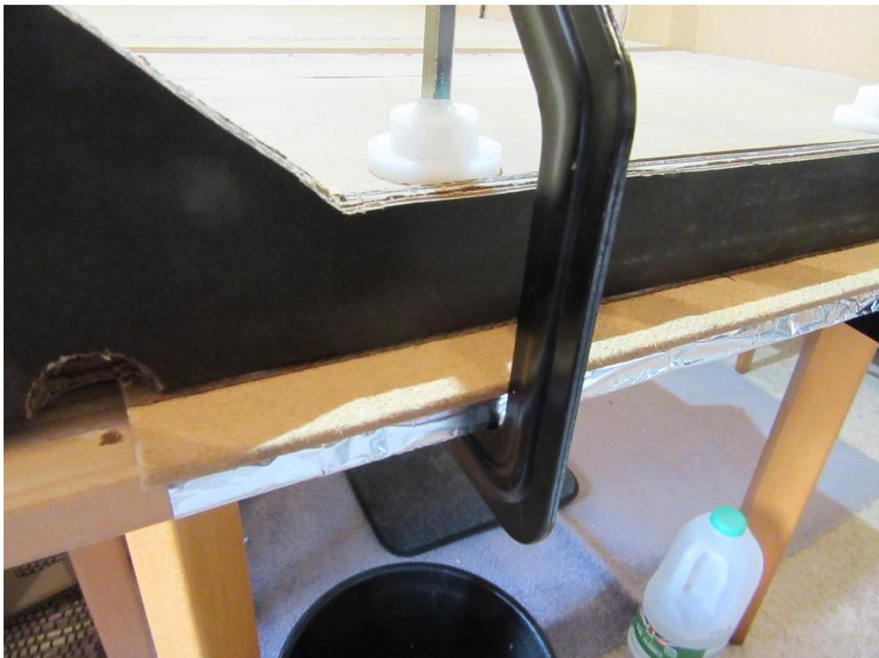
The board is intended join to another (Mark 2!). A simple shelf of hardboard was glued into place for easy alignment. The 2 boards will merely butt together, and may need bulldog clips to hold them together while in use. Time will tell.
